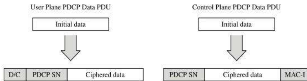
Figure 10.6 PDCP data PDU formats for the user plane and the control plane.
